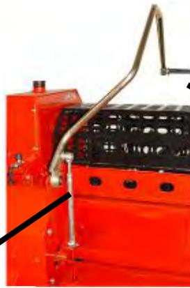
The lever handle can be changed to suit left or right handed users, and the handle can be lifted to the desired height.
