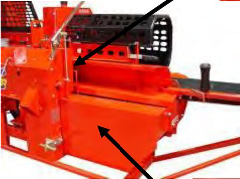
The sensitivity of the input conveyor's movement can be adjusted with the lever mechanism of the valve controlling the conveyor.
