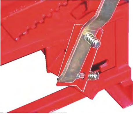
Attach the height adjustment lever for the splitting blade (no. 7 in Figure 2) as shown in the figure. Install the spring that holds the lever in its slot on the outside of the lever, under the head of the bolt. Place the spring that enables the blade's movement under the nut. Tighten the nut so that it applies slight pressure on the spring. Ensure that the spring has enough play. **Note! Does not apply to Easy models.**
