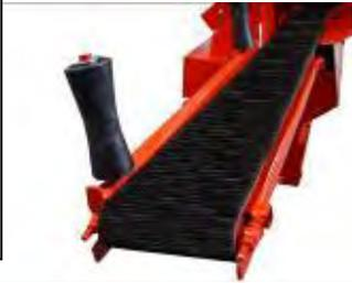
If the belt veers to the side, adjust the belt with the adjustment nut on that side. This will guide the belt to the middle of the frame.
