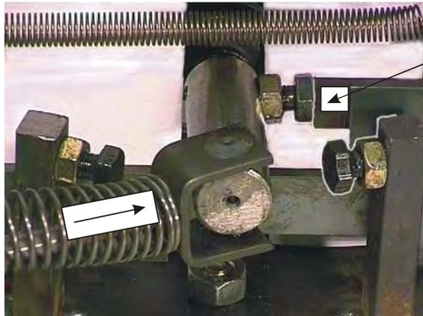
7. The depressed trigger rod stops the jointed lever in the middle position halting the splitting system.
