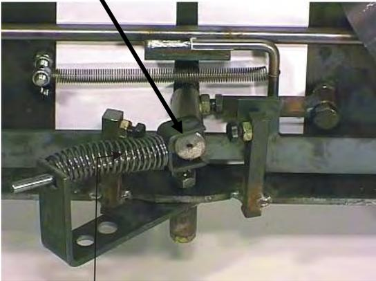
3. After cutting the wood, when the cutting lever is lifted up, the trigger lever is also raised lifting up the trigger rod. When the trigger rod is up, the spring presses the jointed lever to the right enabling the splitting motion to begin.
