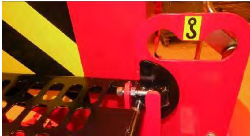
*Figure 4. Lifting points for a chain or strap.*
