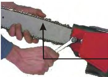
3. Lift the flange and tighten the fastening bolts. Then, lower the guards and lock them in place.
