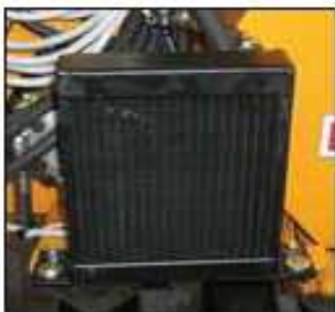
Oil cooler with thermostat (optional TA32-TAR32).
