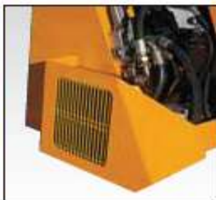
Oil cooler with thermostat (optional TD-TDF).
