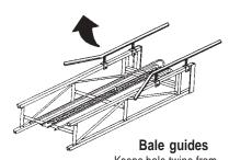
Keeps bale twine from catching and breaking when bales are discharging from a steeply inclined elevator. Prevents bales from tipping and turning and then tumbling out when transferring from an inclined elevator to mow conveyor. Pair of sturdy steel tubes clamp onto sides of inclined elevator on top end.
