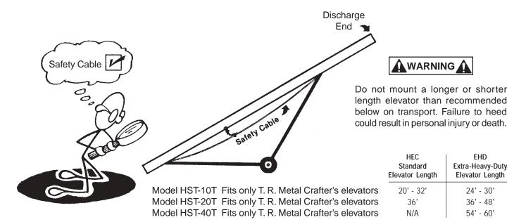
Make sure the safety cable is installed onto transport at the correct location. Refer to Transport Manual for instructions. The safety cable prevents transport from being lowered to an unsafe working position. Failure to install safety cable may result in personal injury or death. Note: Elevator weight should never rest on transport safety cable during normal operation. If safety cable is lost or missing, contact T. R. Metal Crafters, Inc. for free replacement.
