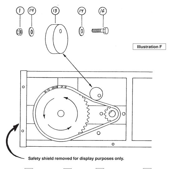
Mount 12" jack pulley <u>#25</u> onto jackshaft <u>#26</u> with screw <u>#23</u>. Tighten set screw <u>#23</u> down onto flat spot on end of jackshaft.
