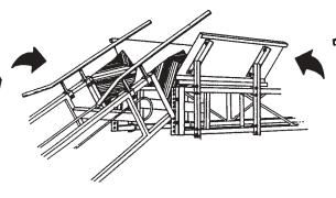
Above drawing illustrates incline elevator assembled to horizontal conveyor, using Bale Guides (model HST-7A), Connector Plates (model HST-17A or 18A) and Bale Arrangers (model HST-16A).
