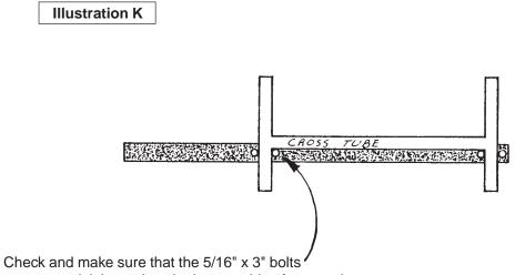
are pressed tight against the bottom side of cross tube.
