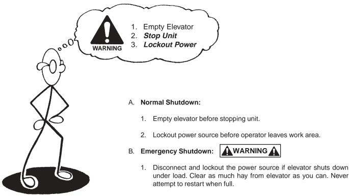
2. Starting the unit under load may result in damage to the elevator. Such damage is considered abuse of the equipment.
