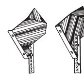
**Connector plates:** Connects incline elevator to horizontal mow conveyor. Prevents bales from turning and tumbling out when transferring.
