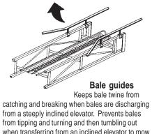
from tipping and turning and then tumbling out when transferring from an inclined elevator to mow conveyor. Pair of sturdy steel tubes clamp onto sides of inclined elevator on top end.
