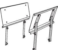
**Bale arrangers:** Directs irregular shaped bales into horizontal conveyor. Made of heavy galvanized steel.
