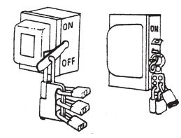
Attaches to main power disconnect switch. Equipment cannot be started until all workmen have removed their personal padlocks.
