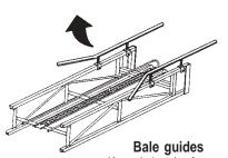
Keeps bale twine from catching and breaking when bales are discharging from a steeply inclined elevator. Prevents bales from tipping and turning and then tumbling out
