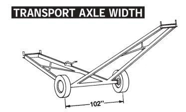
(From center of tire to center of tire - outside width will vary depending on tire width)
