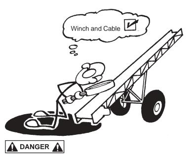
Check winch and cable for condition, security, and operation. There should be at least 3-complete wraps of cable around winch drum in full down position. The cable anchor on the winch drum must be tight.
