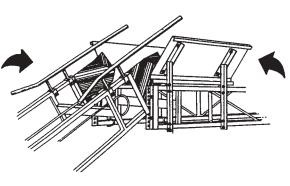
Above drawing illustrates incline elevator assembled to horizontal conveyor, using Bale Guides (model HST-7A), Connector Plates (model HST-17A or 18A) and Bale Arrangers (model HST-16A).
