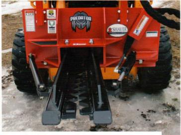
Locking device to lock jaws together to help root and rock removal.
