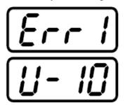
Short circuit on the reed sensor power supply. The device must be immediately switched off with any key and the fault must be removed.
