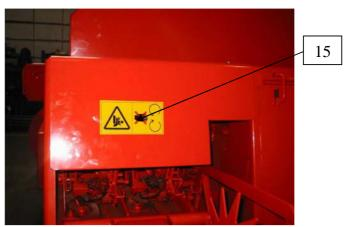
15.Do not get near the needle and knotter zone if the tractor engine is working and PTO shaft is switched on.
