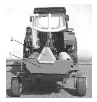
Fig. 24 Bale wrapping machine SIPMA OS 7510 KLARA in the transport positionview from the rear: 1 - casing; 2 - triangular plate
