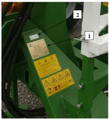
Fig. 21 View of signs 1 - nameplate; 2 - serial number
