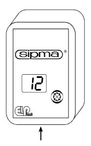
To turn the device on plug the sensor cable into the socket on the bottom of the casing.
