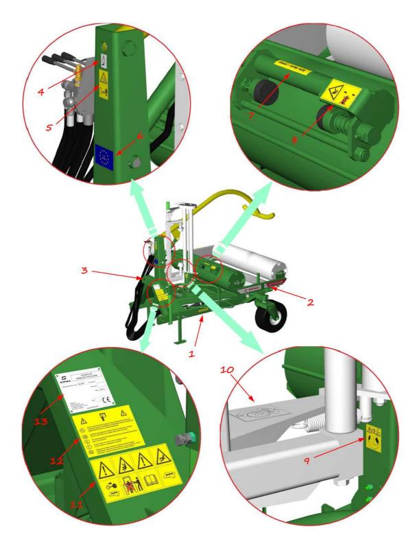
Fig. 20 Arrangement of warning signs on the machine:
