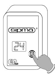
After performing the set number of wraps the display indication must be reset by the button B.
