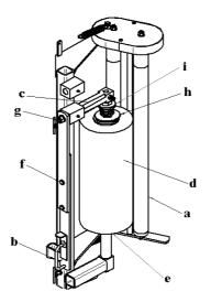
Fig. 29 Mounting 500 mm foil:
