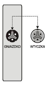
A sensor cable plug has a point (marked on the outside with a longitudinal recess), which must be placed in front of the notch in the socket during insertion.
