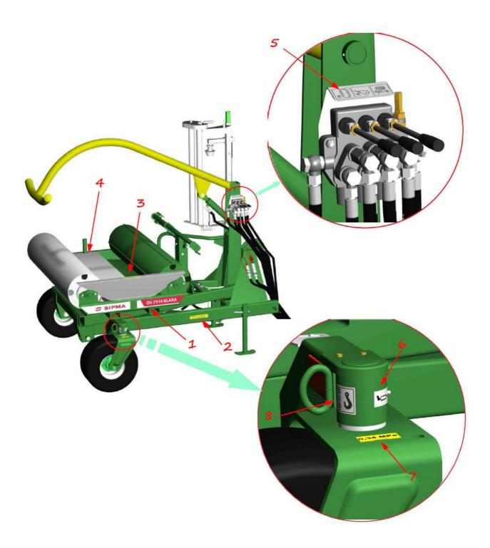
Fig. 19 Arrangement of warning signs on the machine:
