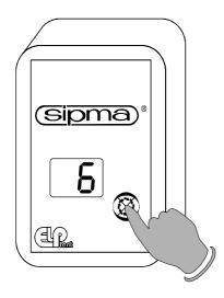
To read the total number of wraps press and hold the button for *10 seconds*.
