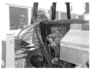
Fig. 27 Connecting hydraulic hoses to the tractor
