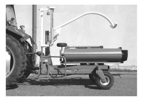
Fig. 25 Bale wrapping machine SIPMA OS 7510 KLARA in the transport position - view from the side
