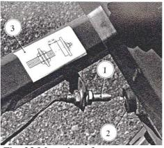
Fig. 23 Mounting of wraps counter 1 - counter sensor; 2 - magnet; 3 - pictogram
