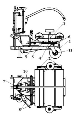
Fig. 37. Greasing points of the bale wrapping machine SIPMA OS 7510 KLARA
