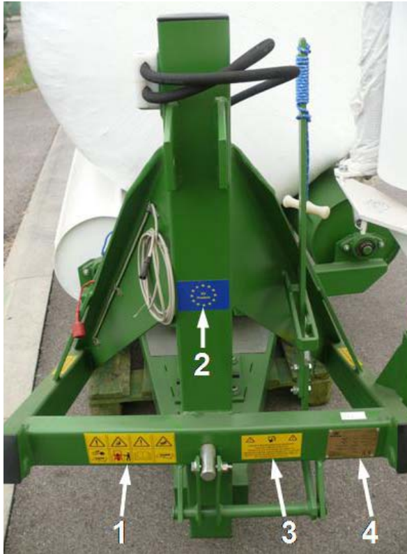
Fig. 17. Arrangement of stickers – view from the front of the wrapping machine: 1 – information pictogram; 2 – EU Product sticker; 3- read the user manual before beginning to operate the machine; 4 – company plate.
