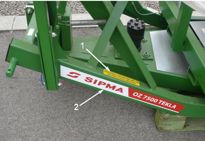
Fig. 15. Arrangement of stickers – view from the left-hand side of the wrapping machine: 1 – information pictogram; 2 – OZ 7500 P sticker.
