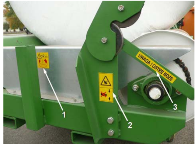
Fig. 18. Arrangement of stickers – view from the back of the wrapping machine: 1 - direction and number of rotations; 2 - Warning! Risk of hand injuries; 3 - warning pictogram.
