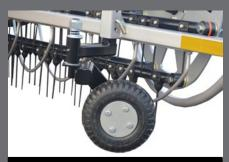
FRONT & REAR GAUGE WHEELS WITH TORSION AXLE SUSPENSION
