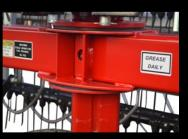
HEAVY-DUTY BASKET PIVOT w/ UHMW SHIMS -SHEAR BOLT PROTECTED
