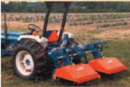
Model FL with 2 heads, clearing row middles during strawberry renovation
