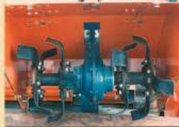
Detail of the blades, model FP. Hubs are easily added or removed to change head width.
