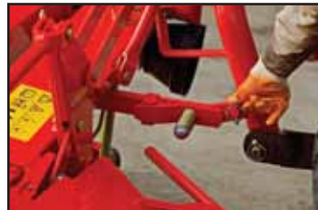
Figure 8- Connect the tension pin and control (2)
