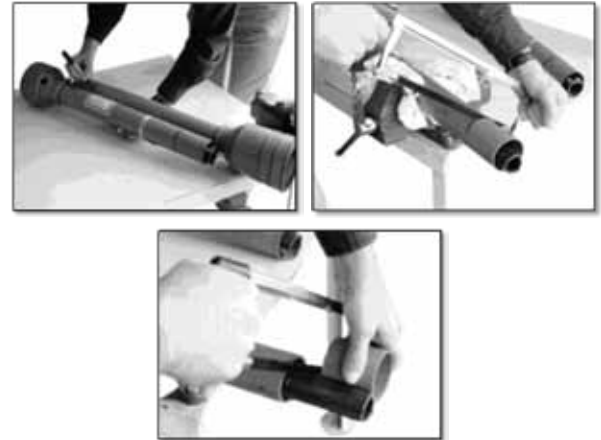
Figure 5- Adjusting the length of the P.T.O shaft to the proper dimension for the tractor.
