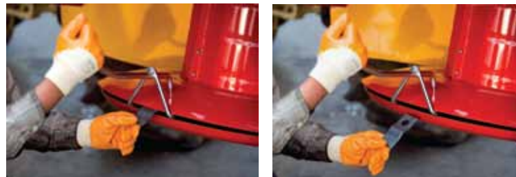
Figure 17- Replacing the knives
