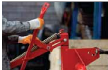
Figure 7- Disconnect the tension spring (1)
