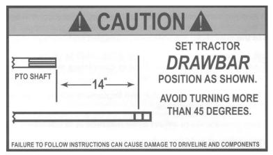
The tractor's drawbar must be set at a distance of 14" from the end of the P.T.O. shaft to the center of the drawbar pin hole. This distance is standard for P.T.O. drives and will maintain a proper relationship for driveline angles and help improve the life of the driveline.
