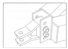
The Hitch is designed to give 3 height positions. The hitch must be set to the proper hitch height to keep the CADDY parallel with the ground.
