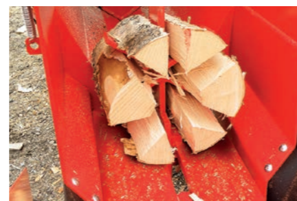
6-way splitting blade available as an accessory.
