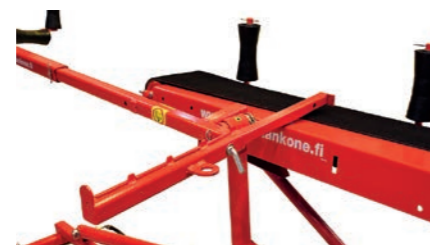
The transport support is pulled out from the arm and over the infeed conveyor.
