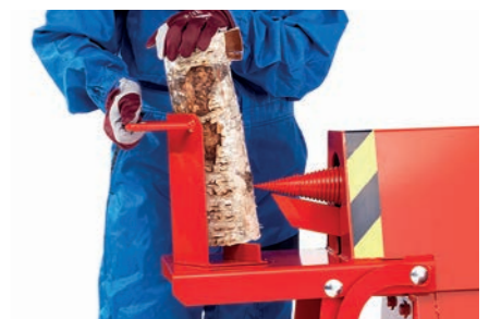
Safe splitting with a steel cone.
