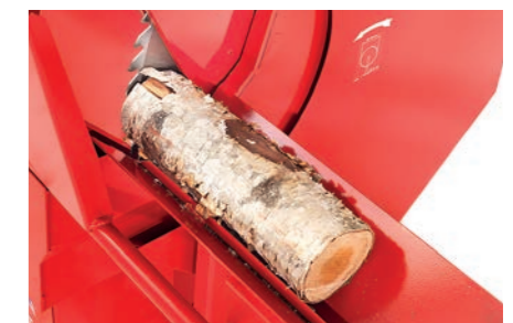
The machine uses a simple cutting cradle in which the log is cut with a hard tipped cutting blade.
