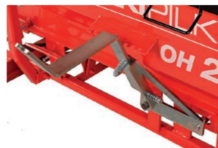
The height of the splitting blade can be adjusted quickly and easily with a manual lever.
