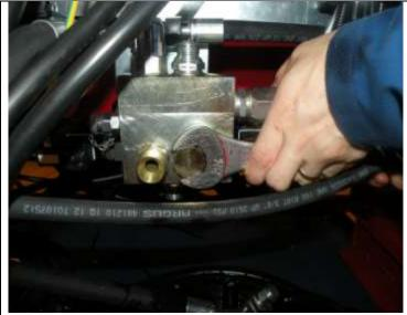
5. Remove the attachment bolts of speed valve and remove the speed valve from the split valve.
