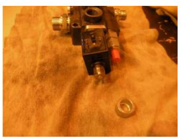
10. Remove the attachment nut of inductor and pull inductor and O-ring off (from both side of shaft).
