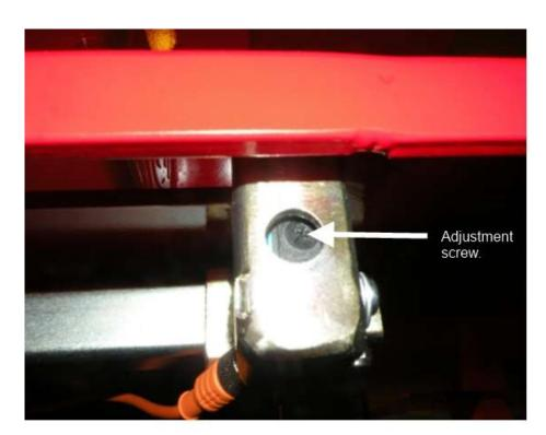
We have also detected some problems with splitting function of HakkiPilke 38 Easy, in which a return movement has been too slow and it has loaded electric motor or tractor too much, because the shaft of split valve hasn't moved fully to return-position. Fix the problem in following manner:
