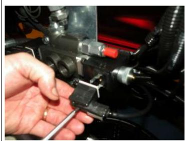
7. Remove the electric plugs of split valve (2 pcs).
