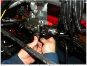
8. Remove the attachment bolts of split valve (2 pcs).
