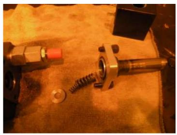
11. Remove the shaft of inductor, springs and washer. (N.B there's only 1 spring on the other side).
