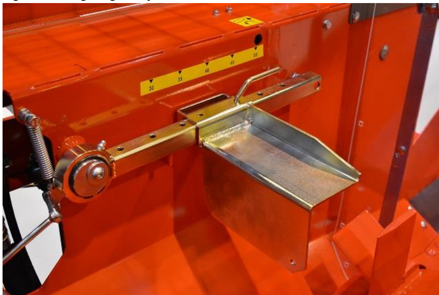
Figure 19. Limiter plate position for smaller logs
