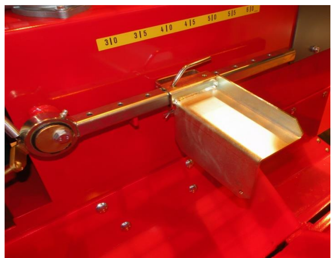
Figure 18. Limiter plate position for small logs
