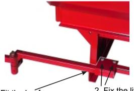
1. Fit the lug for attaching the lifter to the frame of the machine.
