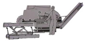
2. Raise the log onto the machine using the lifter.
