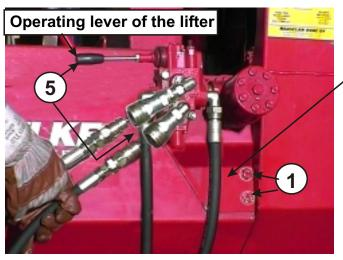
1. Install the valve assembly to the front end of the machine beside the hydraulic motor for the infeed conveyor.
