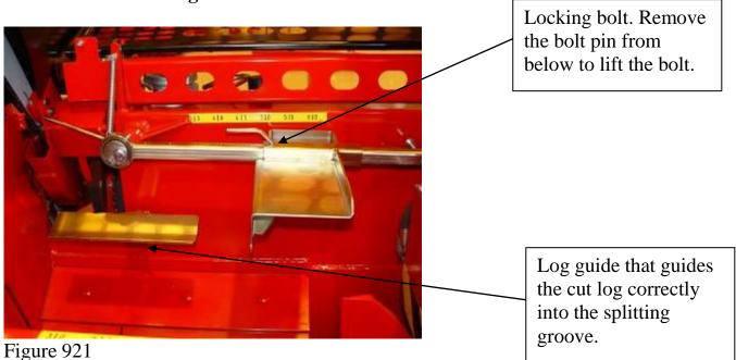
Choose the desired log length from the measuring tape and place the measuring device's front edge to it by lifting the locking bolt and moving the measuring device either forwards or backwards. Remember to replace the locking bolt and its pin.
