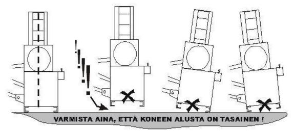
Figure 211 When viewed from the back, the log splitter must stand completely straight!
