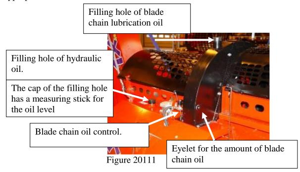
**Note!** The air temperature affects the viscosity of the oil and, therefore, also the amount of oil that is released to the flange.
