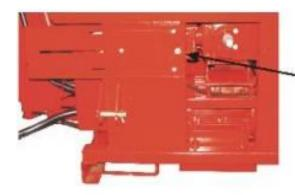
1. Remove the locking bolt of the guard.
