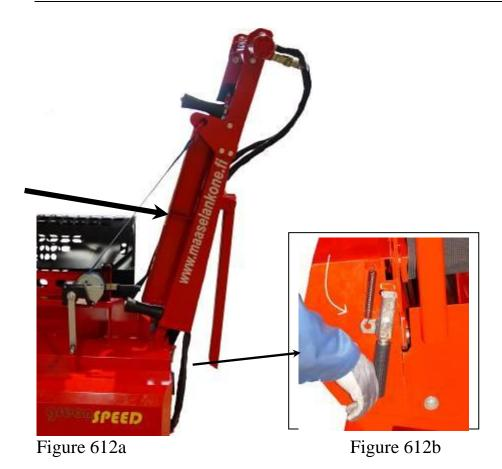
6.1.2 Press the locking handle (Figure 612b) down and then push the output conveyor slowly to the right of the winch until the belt is tight.
