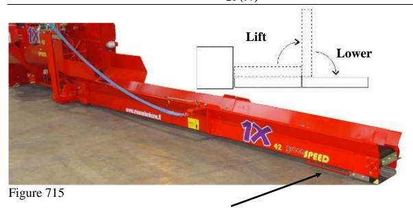
7.1-5 Unfold the output conveyor using handle C according to the figure. Make sure that the conveyor is on level ground and that the winch belt is loose. BE CAREFUL not to get your feet or hands caught in the joint!
