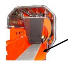
The wood press keeps the logs in place when they are being sawed. Do not put your hand between the wood press roller and the input conveyor belt!
