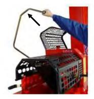
The input conveyor is activated when the cutting lever is moved up from its initial position. Note! In the Easy model, the conveyor can be activated with the control lever B (in Figure 20) by pushing the lever to the up/right position.
