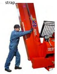
3. Pull the conveyor until the winch strap tightens.
