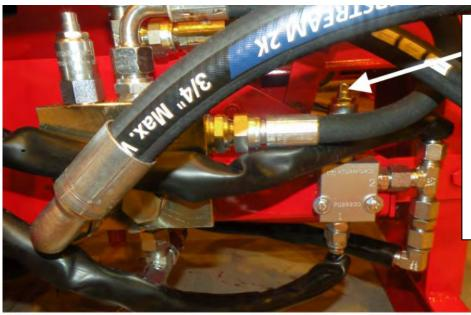
The pressure adjustment cartridge for the cutting flange's downward motion. To increase the pressure, tighten the hex socket screw. To reduce the pressure, loosen the screw. There is no separate design value for the cartridge. The operator should adjust the pressure as necessary.
