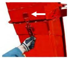
7. Use the winch to adjust the conveyor to the desired inclination, and lock the extension with the lock at the bottom of the conveyor and with a ring pin.
