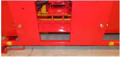
Figure 3. Lifting points for a forklift.
