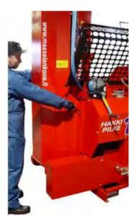
2. Push the conveyor towards the splitter, and release the conveyor lock by lifting the locking bandle
