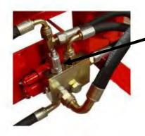
3. Open the locking nut of the acceleration valve's adjustment bolt.
