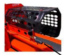
When opening the input conveyor guard, ensure that the locking handle locks the guard in the raised position!
