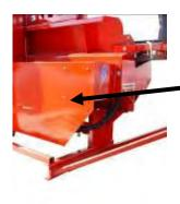
The actual starter box is located behind the splitter, under a protective cover.
