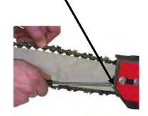
7. Replace the dull blade by reversing the above steps or sharpen the blade by filing it in a vice or sharpening device.
