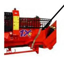
**Note!** The splitting blade can also be removed.
