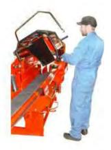
Ensure that the feed conveyor guard is properly locked in the raised position!
