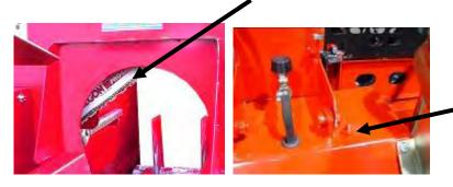
If the blade is not completely raised, tighten the spring pulling the blade by turning its adjustment nut. If the adjustment is not enough, replace the spring.
