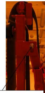
Attach the input conveyor's support (no. 2 Figure 1) to the input conveyor with a bolt.
