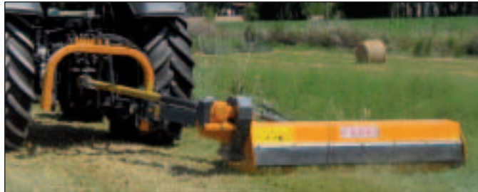
Floating frame: the joint pin on tractor side allows the head system to follow the ground, protecting the arms structure of the parallelogram.
