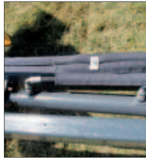
Hydraulic sideshift ram fitted within parallel arms.
