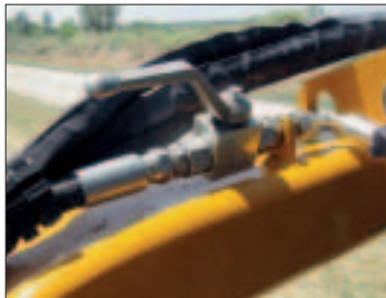
Tap for the locking of the machine in transport position.
