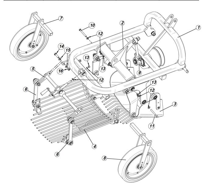
Table 9. Vibrating digger frame with rear discharge
