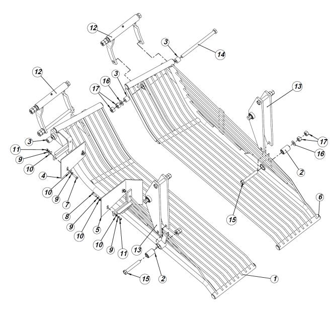
Table 6. Vibrating digger coulter with side discharge
