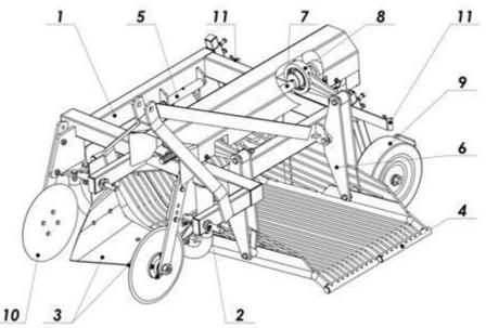
Figure 1. Basic units of vibrating digger: 1 - frame, 2 - studs of three-point suspension system, 3 - topper ploughshares, 4 - sifting hopper, 5 - rockers, 6 - rocker lever, 7 - drive shaft, 8 - connecting rods, 9 - support wheels, 10 - disc coulters, 11 - bracket for the light sign or the triangular sign
