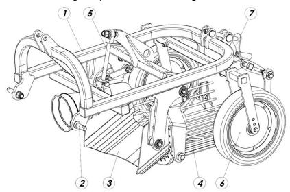
Figure 2. Basic units of the vibrating digger with rear discharge: 1 - frame 2 - three-suspension system studs, 3 - ploughshare, 4 - sifting hopper, 5 - crank mechanism, 6 - support wheels, 7 - mechanism for adjusting the operating angle of the hopper
