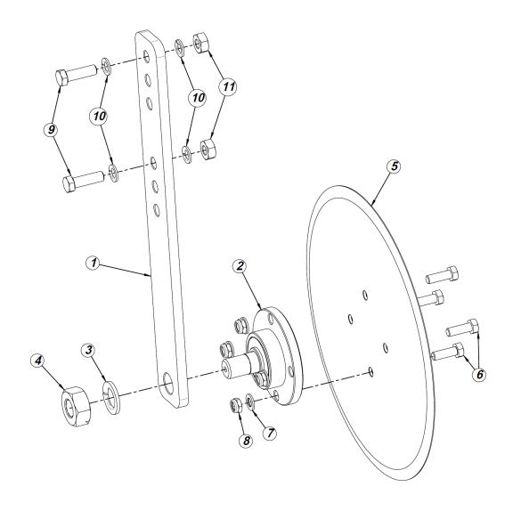
Table 7. Support wheel of the vibrating digger with side discharge
