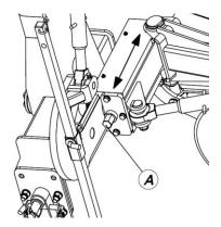
Figure 10. Adjustment of the first furrow screw
