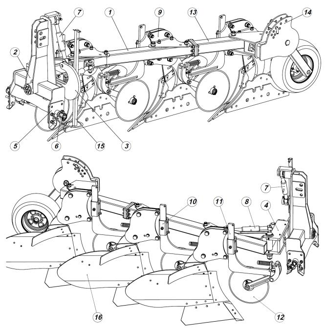
Figure 1. 1-beam plough - general construction: 1 - main frame 2 - three-point suspension system rack, 3 - ledger, 4 - slider, 5 - lower axle overlay 6 - quick hitch beam, 7 - transversal adjustment screw, 8 - longitudinal adjustment screw - alignment, 9 - body saddle, 10 - handle of the coulter or skimmer, 11 - coulter foot, 12 - coulter disc, 13 - frame +1, 14 - support wheel, 15 - support, 16 - body
