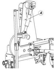
Figure 5. Screw for transversal levelling
