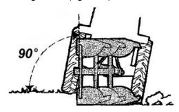
Figure 4. Correct position of the beam
