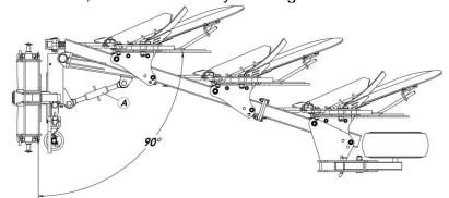
Figure 12. Setting the plough frame after alignment
