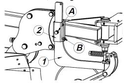
Figure 16. Adjustment of the coulter working depth
