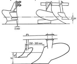
Figure 17. Setting the skimmer in relation to the body
