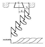
Figure 9. Adjustment of the first furrow width
