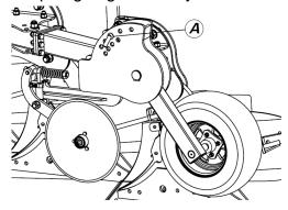
Figure 13. Ploughing depth adjustment
