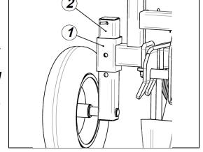
Adjustment of inter-rows, minimum inter-row spacing in the planter is 12cm, and the maximum spacing varies depending on the number of rows planted. For a 3-row planter, the maximum inter-row spacing is **48cm**, for a 4-row it is **32cm** and for a 5-row it is **24cm**.
