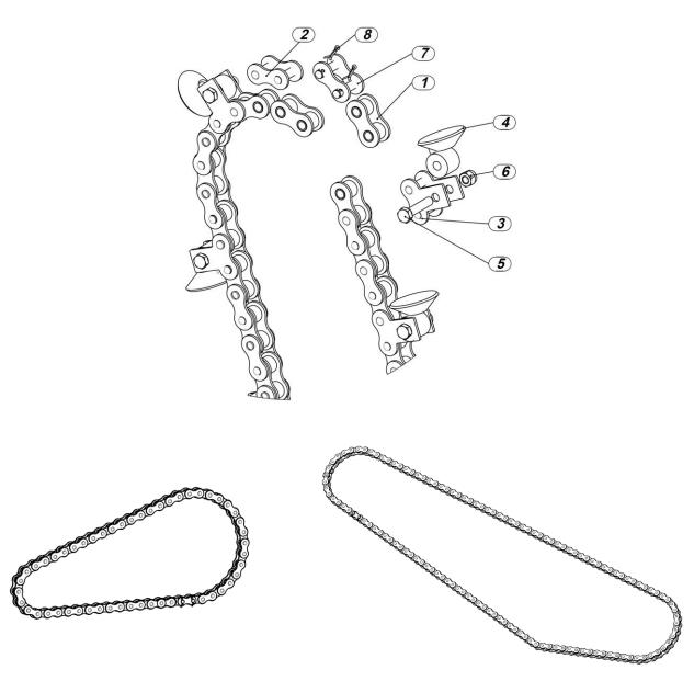
Drive chain L1 inner link 27, outer link 26 + clasp
