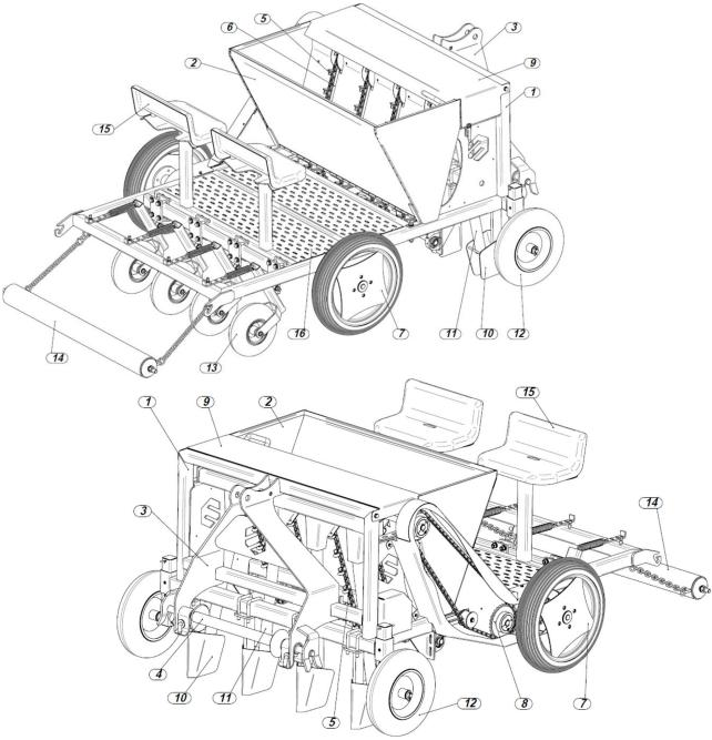
Figure 1. Automatic conveyor 4-row planter: 1 - frame, 2 - tank, 3 - tractor three-point suspension system, 4 - hitching beam, 5 - transport chain conveyor, 6 - chain keeper, 7 - road wheels, 8 - drive sprockets, 9 - drive chain transmission, 10 - markers, 11 - chute pipe, 12 - support wheels, 13 - press wheels, 14 - leveling roller, 15 - seats, 16 - platform
