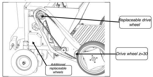
Before starting work, if there is a need to change the planting spacing, select the appropriate replaceable gear wheel together with the Taper Lock sleeve and replace the upper gear wheel. The table below presents the achievable seed planting spacing with appropriate replaceable gear wheels together with the specified types of Taper Lock sleeves.
