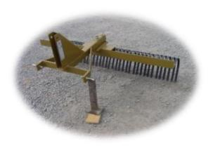
\* COMES ASSEMBLED, ADD A-FRAME AND READY TO USE \* QUICK HITCH READY \* TEETH ARE HEAT TREATED SPRING STEEL \* LOCKING CLAMP TO PREVENT SIDE MOVEMENT OF RAKE TEETH \* ALL BOLTS HAVE STEEL LOCK NUTS TO REDUCE LOOSENING FROM VIBRATION \* COMPACT 3 POINT HITCH A-FRAME AND REPLACEABLE CAT. 1 LIFT ARM PINS \* STAND NOT INCLUDED
