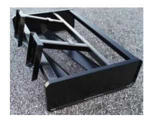
\* SKIDSTEER STYLE HOOK UP \* RECYCLES GRAVEL BY TURNING, MIXING, SIFTING, AND LEVELING WITH NO WASHBOARD EFFECT ON UNPAVED ROADS \* DIGGING OF THE DUAL CUTTING EDGES CAUSES GRASS AND DEBRIS TO FLOW THROUGH EVENLY \* DUAL CUTTING EDGES ARE ANGLED FOR CONSTANT DOWN PRESSURE RESULTING IN BETTER CUTTING AND LEVELING
