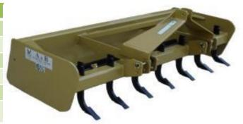
\* ALL WELDED, NO ASSEMBLY REQUIRED \* CAT. 1/2 COMBINATION HITCH \* FLOATING OR LOCKED REAR MOLDBOARD \* SCARIFIER SHANKS ARE ON 11" CENTERS \* FRONT MOLDBOARD ROLL FORMED FOR ADDED STRENGTH AND IMPROVED SOIL FLOW \* REAR MOLDBOARD IS DOUBLE FORMED FOR ADDED STRENGTH \* SCARIFIER SHANKS ARE QUENCHED AND TEMPERED WITH 3 DEPTH SETTINGS
