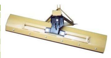
\* QUICK HITCH READY \* COMES ASSEMBLED INSTALL A-FRAME AND READY TO USE \* 1/4"THICK MOLDBOARD DOUBLE FORMED FOR ADDED STRENGTH \* DITCHING BLADE ROTATION ALLOWS ANGLING OF 15 AND 30 DEGREES \* SLIDER STYLE ALLOWS BLADE TO OFFSET RIGHT OR LEFT UP TO 16" \* REINFORCED BLADE ROTATION ASSEMBLY WITH 5 POSITIONS FORWARD AND REVERSE \* REPLACEABLE CAT. 1 LIFT ARM PINS
