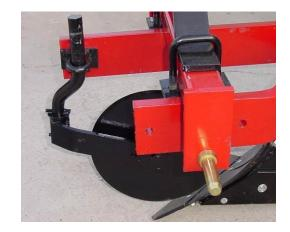
Gauge Wheel is shipped assembled and has only to be bolted to the Short Bar (P-11) using the Clamp Assembly (P-63 & P-64) with lock washers and nuts provided as shown in the picture below.
